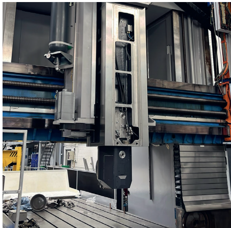
Completely new drive unit including milling head mounted on the existing GRÄSSNER gantry.
